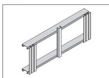
Fix the bottom row of expressed panels allowing a 15mm overlap of the Multiboard Clad Seal 50mm CS-3/25. Leave the top row of fasteners in the Multiboard panels loose to facilitate the insertion of the backing strip to the board.
