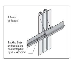
After the backing strip is in position, the top row of fasteners need to be tightened to draw the **eXBound** and backing strip against the top hat, completing the seal.
