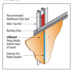
The backing strip joint has been designed to overlap whilst retaining a flush fit behind the board.
