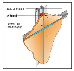
Position the **eXBound** sheet ensuring all joints are 10mm, then fasten the sheet to the top hats using the appropriate fasteners.
