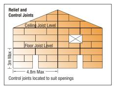
Form a 10mm gap between the **eXBound** sheets and fill with flexible fire rated acrylic sealant according to the FRL required.
