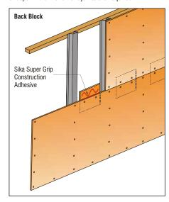
Joints between **eXBound** panels are to be back blocked using a 200mm section of Multiboard offcuts, glued and screwed behind the sheet edges to provide support across the joint. **Sika Super Grip** construction adhesive is recommended or similar.
