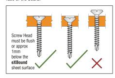
Fasteners must not be overdriven, as this can reduce the holding capacity of the sheet.
