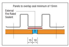
Prepare the backing strip for installation by applying recommended Multiboard Clad Seal to the bottom (9mm) edge of the backing strip or by applying the sealer to the top edge of the **eXBound** sheet.
